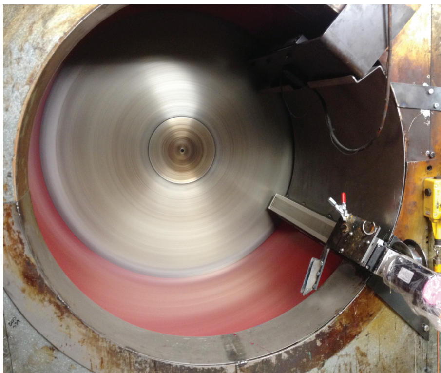
An automated casting arm in this centrifuge drum has helped to advance Urethane's manufacturing process.
